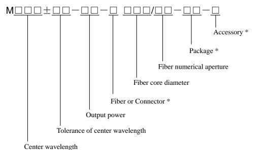
\* Accessory: T – TE cooler, A – Aiming laser, P – Monitor photodiode, K – Fiber connector detector
