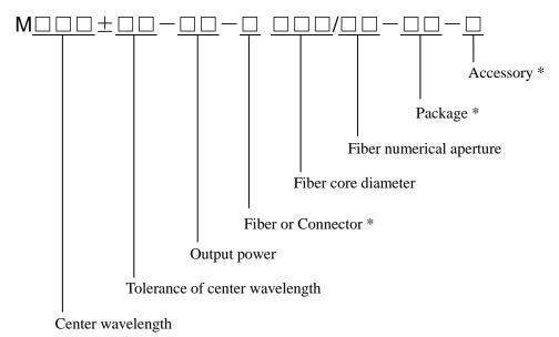
\* Accessory: T – TE cooler, A – Aiming laser, P – Monitor photodiode, K – Fiber connector detector
