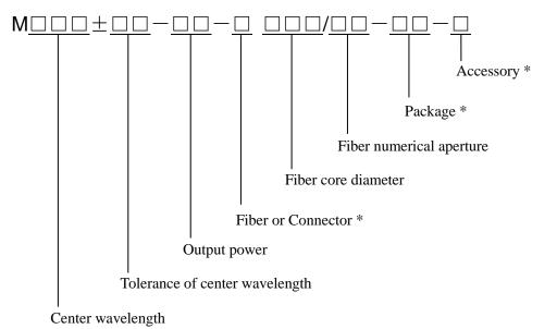
\* Accessory: T-TE cooler, A-Aiming laser, P-Monitor photodiode, K-Fiber connector detector
