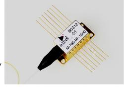
power from a 14-pin butterfly package with  $100\mu m$  fiber core. All modules come standard with an internal thermistor, TEC, and photodiode. Axcel's trademark laser chip design creates un-measurable degradation and long lifetimes that make our chips among the most reliable in the industry today. Our 785nm multi mode line serves a broad range of applications including Raman Spectroscopy, laser pumping, and medical laser therapy.
