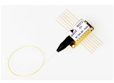
continuous output power from a 14-pin butterfly packaged 100 um fiber. All modules come standard with an internal thermistor, TEC, and photodiode. Axcel's trademark laser chip design creates unmeasurable degradation and long lifetimes that make our chips that are among the most reliable in the industry today. Our multi mode line serves a broad range of applications including solid state pumping, fiber lasers, material processing, graphics, medical, and defense.
