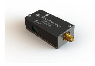
A compact Acousto-Optic Frequency Shifter featuring a generous active aperture, low power 350mW 80MHz supply requirement and high diffraction efficiency, this device is ideal for use in heterodyne interferometric systems, particularly laser Doppler velocimetry and has been designed to facilitate double pass configuration.
