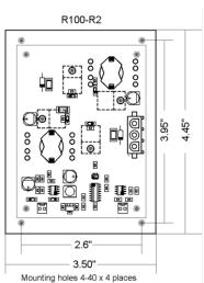
Dimensions of the driver board with integral mounting plate.
