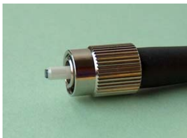
figure 1: SAM chip on FC/PC connector end face
