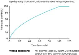
The special core composition of the PS series fiber enables
