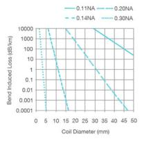
The fibers are available in a range of Numerical Apertures (NAs) from 0.13NA up to 0.31NA. Low NA fibers are designed for low attenuation applications where long lengths of fiber are used in a straight deployment state, for example in Distributed Temperature Sensing (DTS) systems. High NA fibers allow dramatically reduced bend losses for coiled deployment states, for example in coiled seismic/acoustic sensors.
