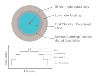
Fibercore's triple-clad erbium/ytterbium doped fibers (TC1500Y) are designed as single-mode, high-power CATV and telecommunications amplifier fibers. The TC1500Y(6/125)HD offers a smaller Mode Field Diameter (MFD) for higher efficiency levels at output signal power around 1W. The TC1500Y(11/125)HD is designed for output signal power at 5W and above.
